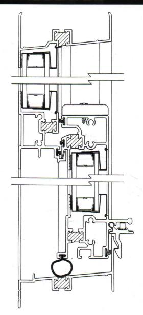
Heavy .062 aluminum extrusion with structural thermal barrier for maximum strength and insulation.
